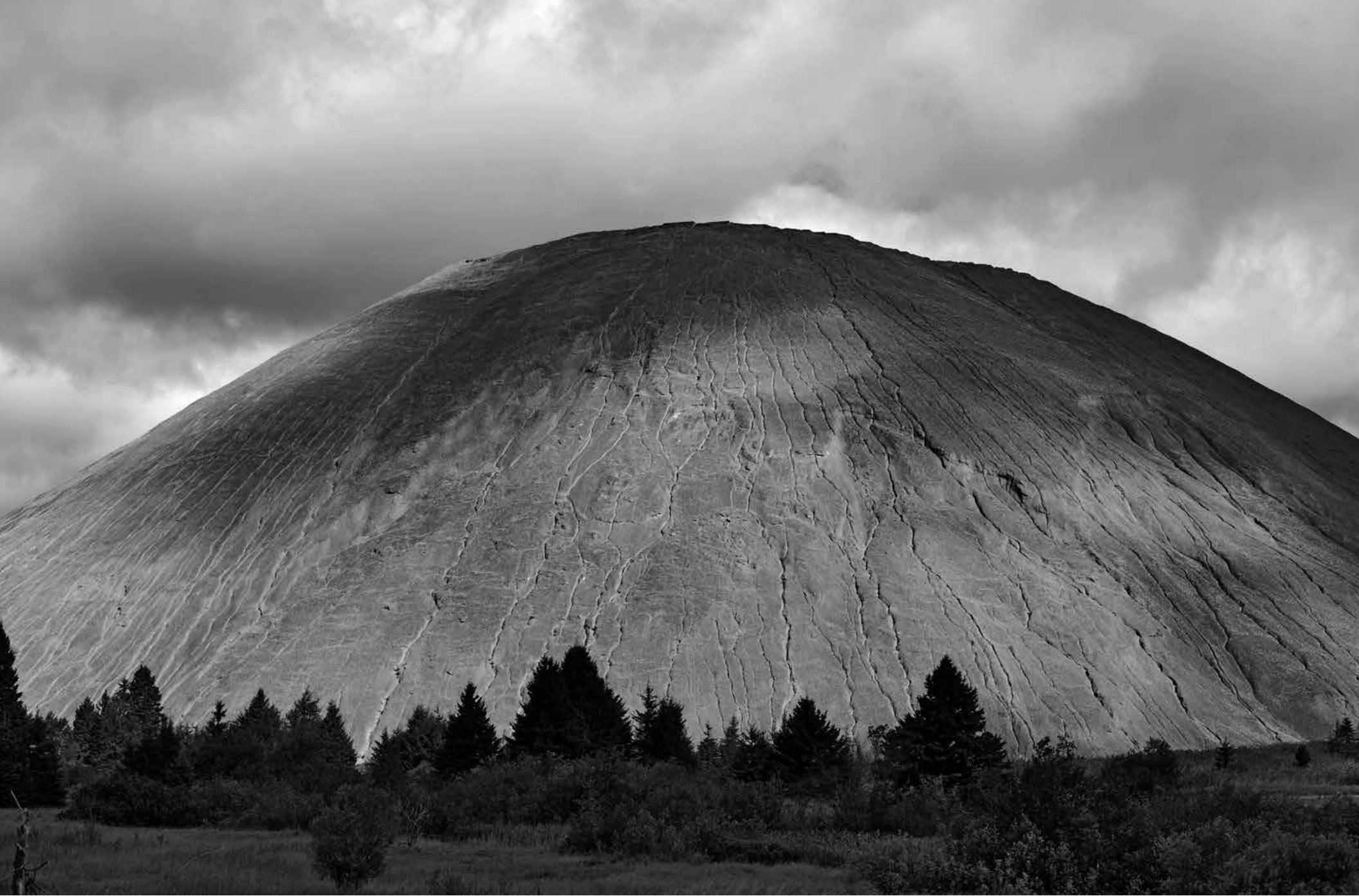
Asbestos tailings from the mining of chrysotile asbestos, a.k.a. white asbestos, seen in the city of Thetford Mines in Quebec, Canada.
